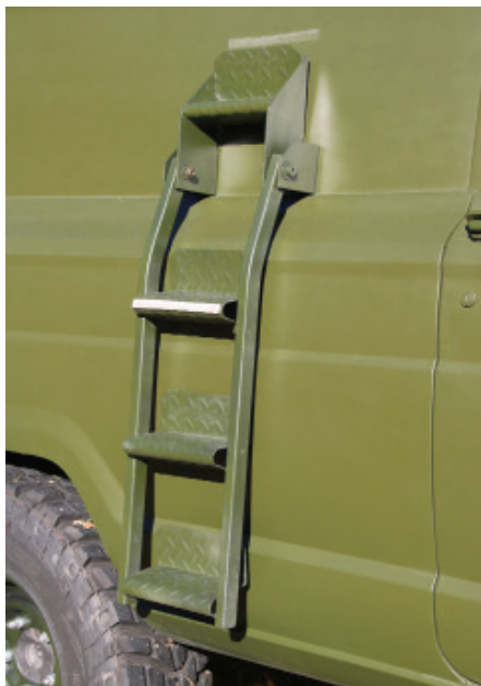
A folding ladder provided access to the roof platform.
