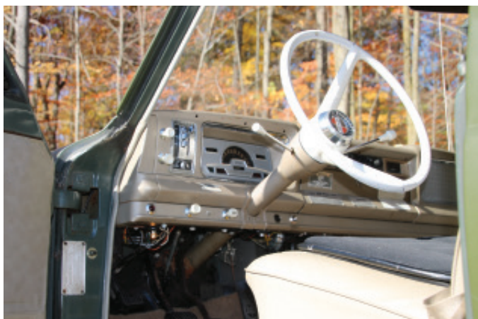
Basically a converted civilian vehicle, the Jeep J100 AV was delivered to the Army with a complete, civilian interior.
