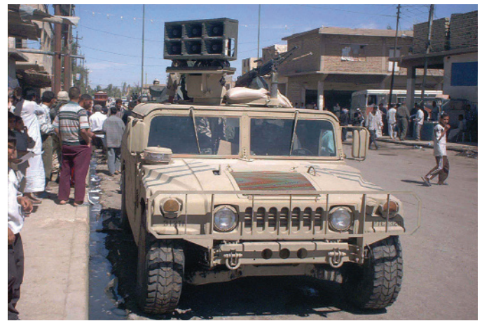
Today, PSYOP units continue to use audio-visual equipment to carry out their missions. It is not unusual to see current audio visual platforms and speakers mounted on variants of the M998 HMMWV series.
