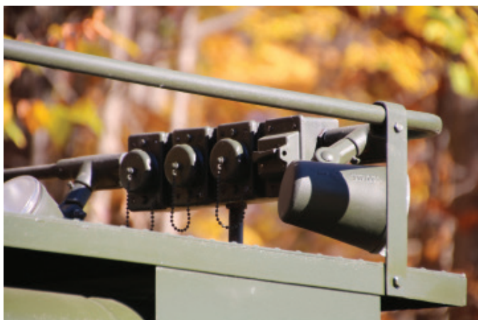
Roof electrical connections and lights were mounted on the guard rail surrounding the roof platform.
