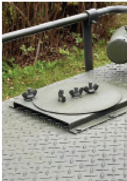
Loud speakers could be affixed at one of the special mounting points located on the roof platform.
