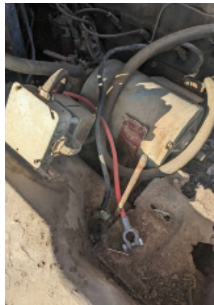
A PTO-driven, 120-volt generator provided AC-power to operate the vehicle's 16 mm movie projector, audio speakers, magnetic tape player, and phonograph.
