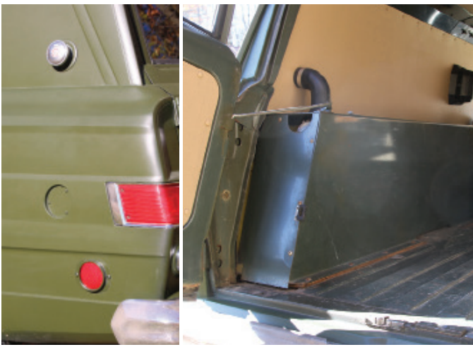
Second fuel tank and modified filler location are distinctive, identifying attributes of a specialized J100 Panel Delivery AV truck.
